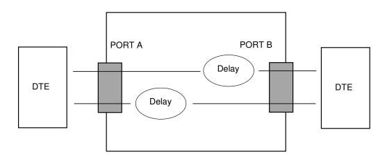
The error-injection facility allows typical line characteristics and fault conditions to be simulated, in conjunction with delay and clock generation facilities. Errors are injected in the local data stream just prior to output:
