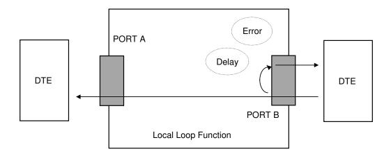
The Remote Loop mode routes the data back to the local port in the same way but this time via the delay and error-injection facilities:
