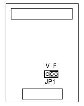
JP1 selects Fixed or Variable interface signal output. It should be left in the 'F' position when fitted in Simulator 2.
