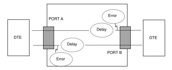
Data loop facilities are provided to allow the operator to verify the integrity of the DTE equipment and cabling connected to each port. The Local Loop mode routes data from TXD back to RXD at the local port without being subject to delay or error conditions:
