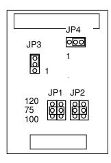
JP1 and JP2 are double-jumpers for selecting the G.703 receive termination impedance and must be set the same, in one of the three positions indicated. For E1 long-haul, select 75ohms (Coax) or 120ohms (UTP). For T1, select 100ohms.
