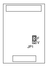
JP1 selects Fixed or Variable interface signal output. It should be left in the 'F' position when fitted in Simulator 2.
