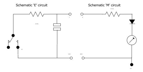
The E&M signalling return paths must be connected externally. This can be accomplished by connecting the EREF lead to the PABX frame ground with a good cable.
