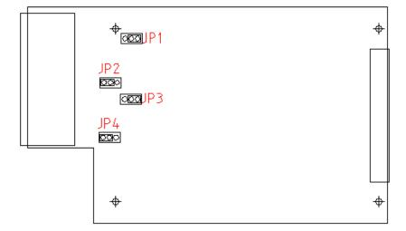
The next diagram shows the FXO variant with the jumpers fitted in their default positions:
