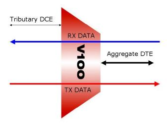
NOTE: By convention, the Receive Clock "RXC" is defined as "the clock associated with the direction of data flow from aggregate to tributary" and the Transmit Clock "TXC" as "the clock associated with the direction of data flow from tributary to aggregate". This assumes that aggregate ports are normally DTE presentation and tributaries are normally DCE, so for an aggregate, RX data is input and TX data is output whereas for a tributary, RX data is output and TX data is input.
